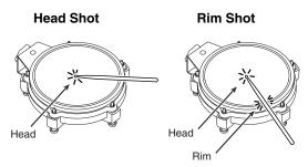
To play the sound assigned to the head, hit only the head. To play a rim shot, you must **strike both the head and the rim of the pad simultaneously**.
