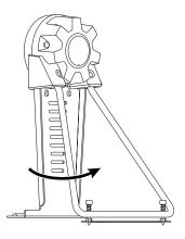
Use the tuning key supplied with the FD-8 to tighten the screws removed in Step 1 so that the stand is firmly secured.
