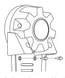
2. Pull out the stand in the direction indicated by the arrow until it is fully extended.
