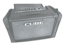
2. Tighten the strap on the top of the carrying case to secure the case and the unit in place.
