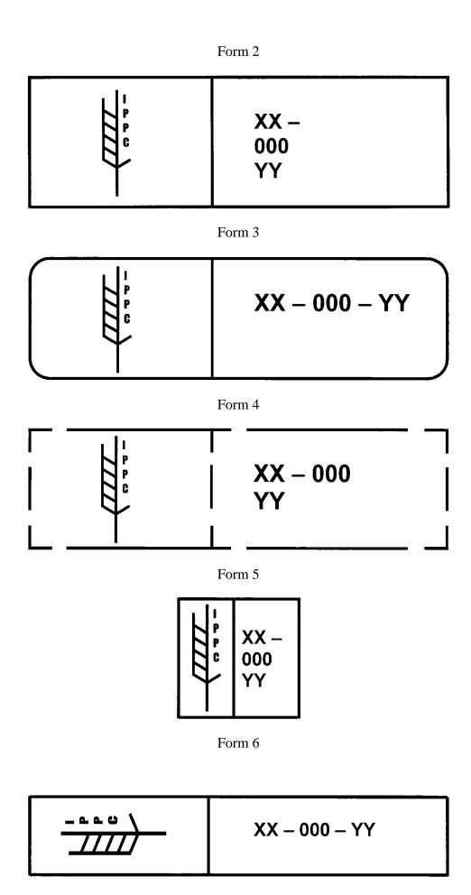
Fig. Marking Forms for Wood Packaging and Fixing Materials
